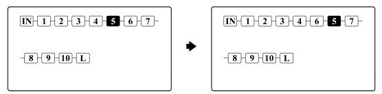
Select the Loop 5 and press switch #7 to move the right.
