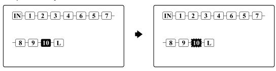
Select the Loop10 and press and hold the switch #6 to set to the carry-over.
