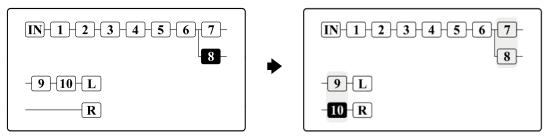
3. Select the loop 8 and press and hold Switch #4 to move it to the lower line.
